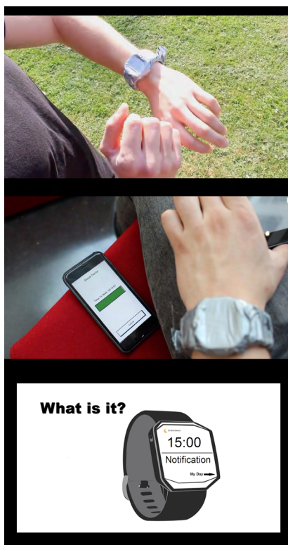
Figure 5. (Case study 4) Stills from student-produced video demonstrating the functionality of a smartphone app which interacts with a smart watch in a lo-fi prototype.
